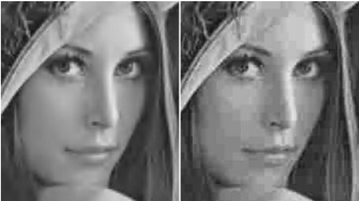
Fig. 23. Lena image ( 512 \times 512 ) decompressed at 0.25 b/pixel using JPEG2000 (left) and JPEG (right). A cropped and zoomed portion of the fully decompressed image is displayed here.
