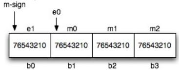
Fig. 5C-18. IEEE 754 single precision real, most significant byte first
