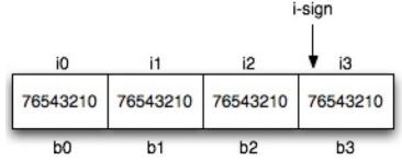
Fig. 5C-2. Signed 4-byte integer, least significant byte first
