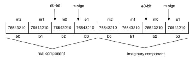
Fig. 5C-20. Single precision complex, least significant bytes first.
