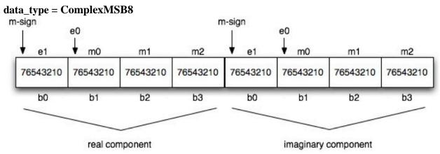
Fig. 5C-22. Single precision complex, most significant bytes first.
