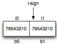
Fig. 5C-3. Signed 2-byte integer, least significant byte first
