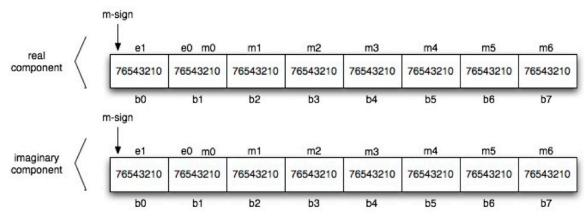
Fig. 5C-21. Double precision complex, most significant bytes first.
