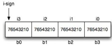
Fig. 5C-10. Signed 4-byte integer, most significant byte first
