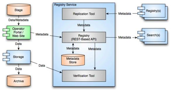
Figure 4: Registry Service Architecture (with Storage)
